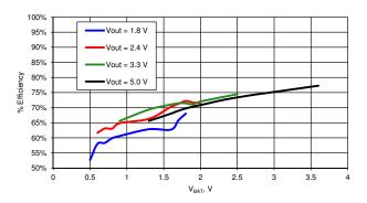
Figure 11-13. Efficiency vs  $V_{BAT}$ ,  $L_{BOOST}$  = 22  $\mu H^{[42]}$
