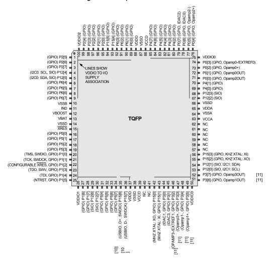
Figure 2-6. 100-pin TQFP Part Pinout
