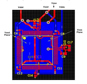
Figure 2-8. Example PCB Layout for 100-pin TQFP Part for Optimal Analog Performance
