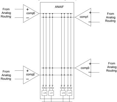
Figure 8-5. Analog Comparator
