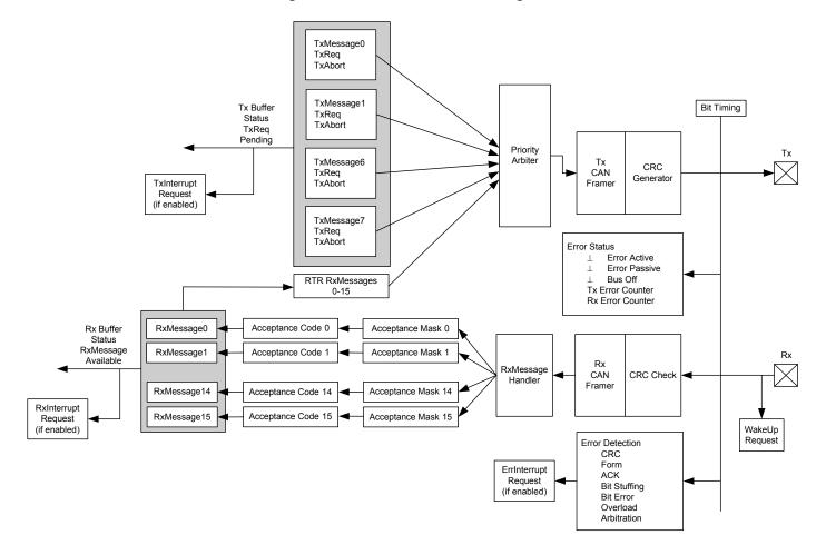
Figure 7-15. CAN Controller Block Diagram
