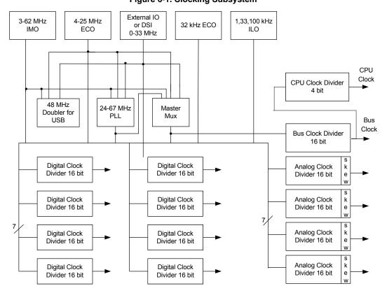
Figure 6-1. Clocking Subsystem
