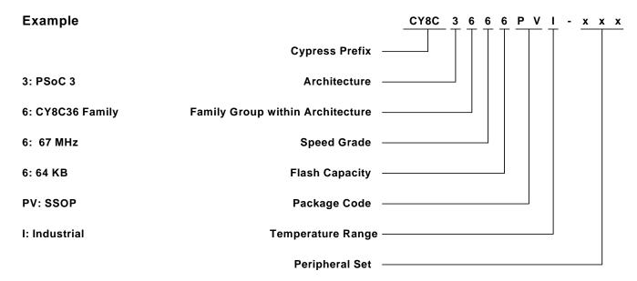
Tape and reel versions of these devices are available and are marked with a "T" at the end of the part number.
