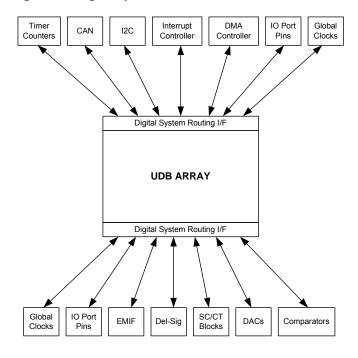
Interrupt and DMA routing is very flexible in the CY8C36 programmable architecture. In addition to the numerous fixed function peripherals that can generate interrupt requests, any data signal in the UDB array routing can also be used to generate a request. A single peripheral may generate multiple independent interrupt requests simplifying system and firmware design. Figure 7-10 shows the structure of the IDMUX (Interrupt/DMA Multiplexer).
