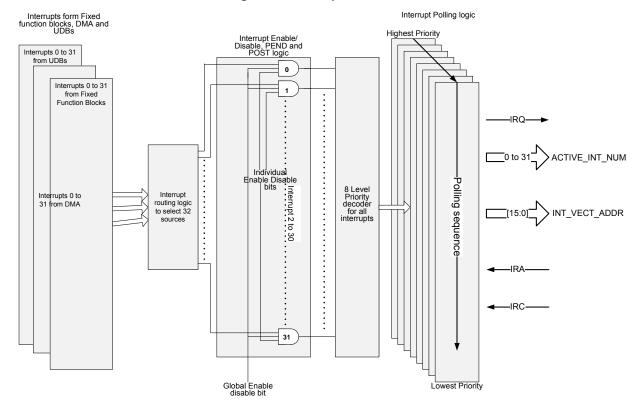
Figure 4-3. Interrupt Structure
