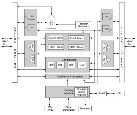
Figure 8-1. Analog Subsystem Block Diagram
