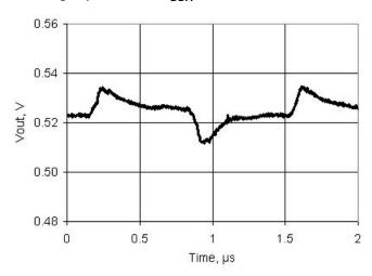
Figure 11-61. VDAC Voltage Noise, 1 V Mode, High speed mode,  $V_{\text{DDA}}$  = 5 V
