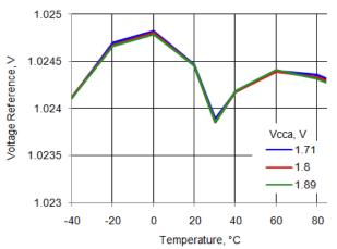
Figure 11-35. Voltage Reference Long-Term Drift
