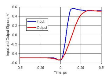
Figure 11-32. Opamp Step Response, Falling
