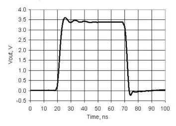
Figure 11-21. SIO Output Rise and Fall Times, Slow Strong Mode,  $V_{\rm DDIO}$  = 3.3 V, 25 pF Load
