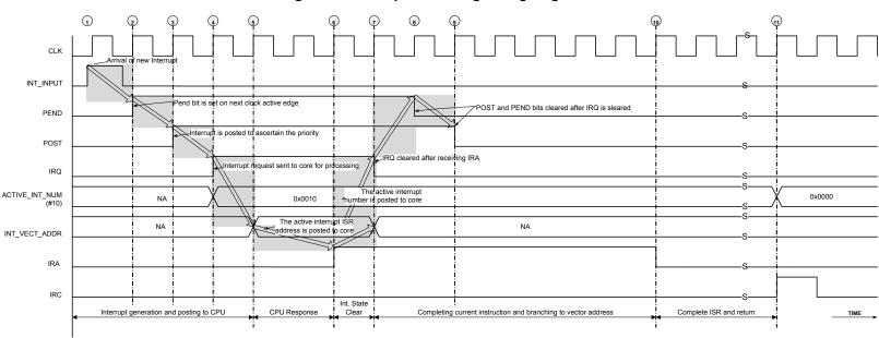
Figure 4-2. Interrupt Processing Timing Diagram
