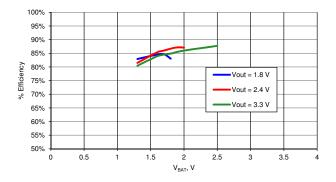
Figure 11-12. Efficiency vs  $V_{BAT}$ ,  $L_{BOOST}$  = 10  $\mu H^{[42]}$
