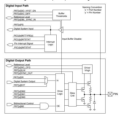
Figure 6-10. SIO Input/Output Block Diagram
