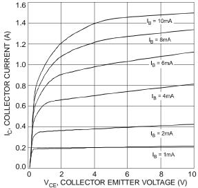
ig. 2 Typical Collector Current vs. Collector Emitter Voltage
