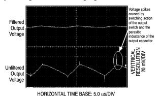
Figure 25. Output Ripple Voltage Waveforms
