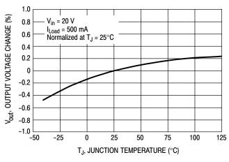
Figure 2. Normalized Output Voltage
