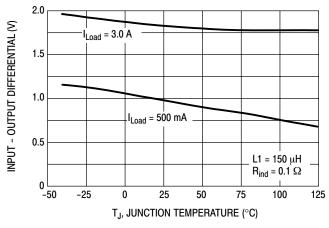
Figure 4. Dropout Voltage
