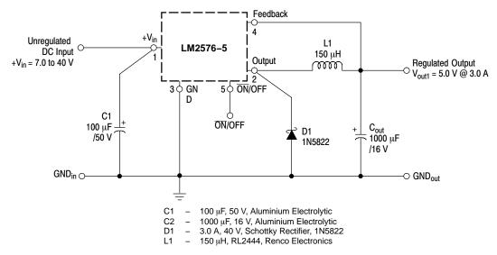
Figure 35. Schematic Diagram of the LM2576-5 Step-Down Converter
