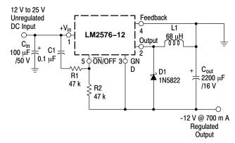
Figure 27. Inverting Buck-Boost Regulator with Delayed startup
