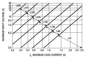
60 H1000 H680 H470 -H330 H220 H150 40 MAXIMUM INPUT VOLTAGE (V) 20 15 12 10 9.0 8.0 L47 0.3 0.4 0.6 1.0 1.2 2.0 2.5 3.0 IL, MAXIMUM LOAD CURRENT (A)
