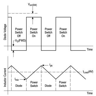
Figure 17. Buck Converter Idealized Waveforms
