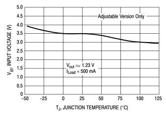
Figure 11. Minimum Operating Voltage
