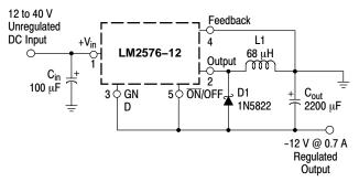
Figure 26. Inverting Buck-Boost Develops -12 V
