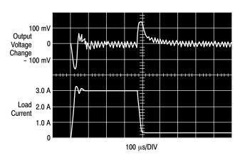
Figure 14. Load Transient Response
