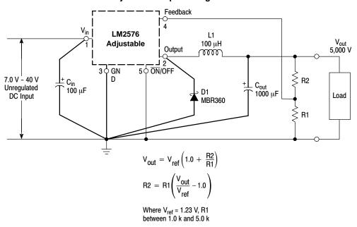
Figure 15. Typical Test Circuit
