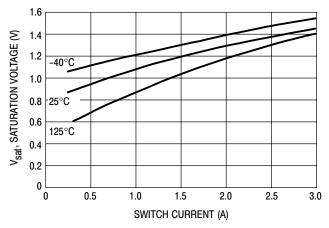
Figure 9. Switch Saturation Voltage
