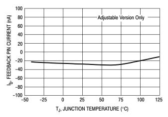
Figure 12. Feedback Pin Current
