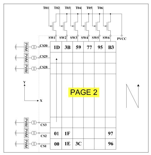
Figure 10 Scaling Register
