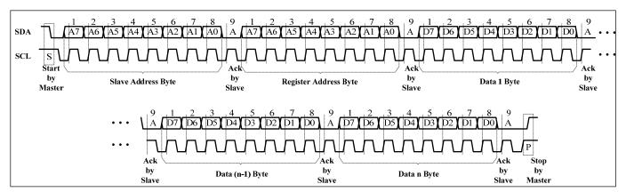
Figure 7 Writing to IS31FL3742 (Automatic Address Increment)
