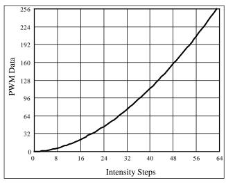
Figure 14 Gamma Correction (64 Steps)
