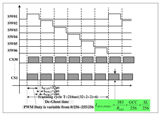
Figure 12 Scanning Timing
