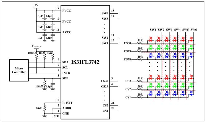
Figure 2 Typical Application Circuit (RGB Color: 10x6)
