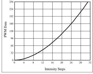
Figure 13 Gamma Correction (32 Steps)
