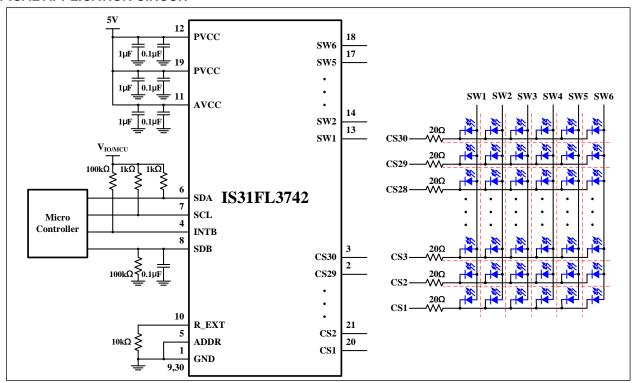
Figure 1 Typical Application Circuit (Single Color: 30x6)
