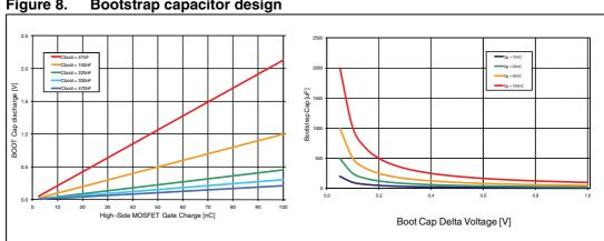
Figure 8. Bootstrap capacitor design
