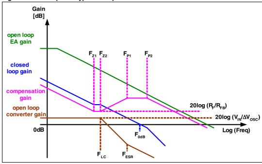
Figure 10. Example of Type III compensation
