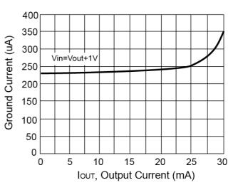
Figure 2. Ground Current vs. Output Current
