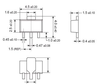
SUGGESTED PAD LAYOUT (Unit: Millimeters)
