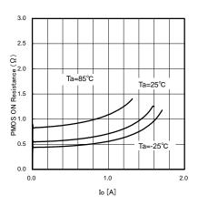
Fig.17.PchFET ON resistance Io property [VCC=5.0V]
