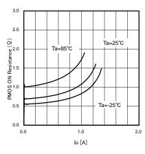
Fig.15.PchFET ON resistance Io property [VCC=4.0V]
