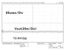
Fig.47 Output ripple 4 (VCC=12V, Io=170mA)
