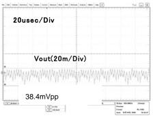
Fig.45 Output ripple 2 (VCC=12V, Io=100mA)
