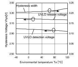
Fig.9. UVLO threshold temperature property
