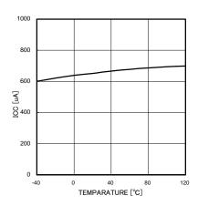
Fig.19. Circuit current temperature property
