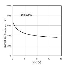
Fig.13. Pch FET ON resistance power supply property
