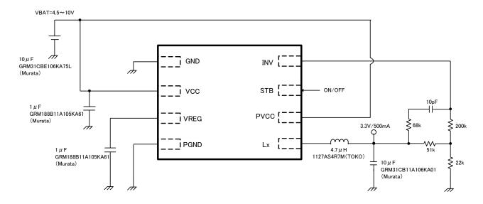
Fig.21 Reference application diagram1
