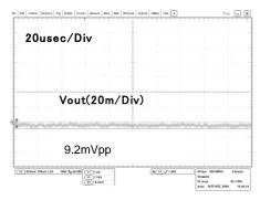
Fig.46 Output ripple 3 (VCC=12V, Io=140mA)
