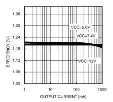
Fig.34 Load regulation (VOUT = 1.2 V)
