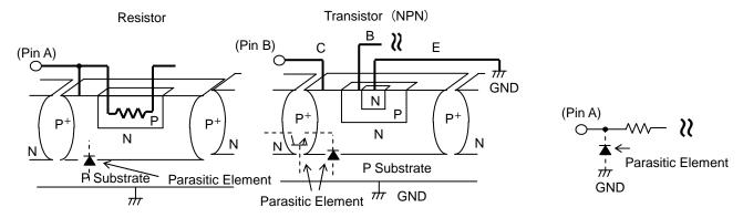
Fig.53 Example of simple structure of Bipolar IC
