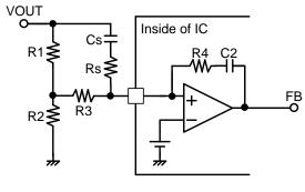
Fig.51 Example of phase compensation setting
