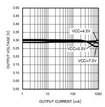
Fig.23 Load regulation (VOUT = 3.3 V)
