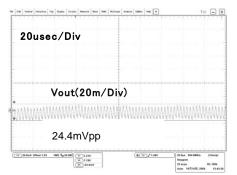
Fig.44 Output ripple 1 (VCC=12V, Io=40mA)
