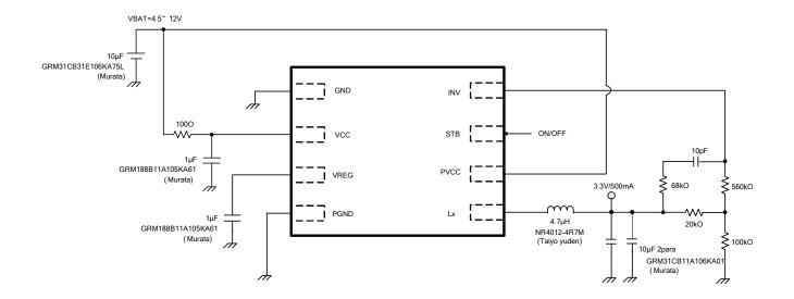
Fig.32 Reference application diagram2
