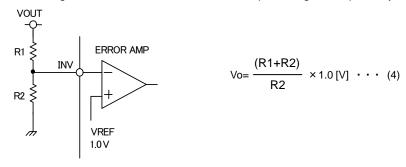
Fig.50 Setting of voltage feedback resistance
