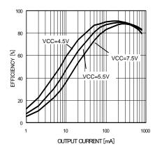
Fig.22 Power conversion efficiency (VOUT = 3.3 V)
