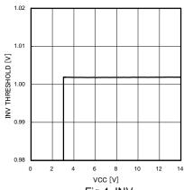
Fig.4. INV threshold power supply property
