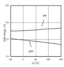
Fig.18. STB threshold temperature property
