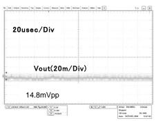
Fig.48 Output ripple 5 (VCC=12V, Io=900mA)
