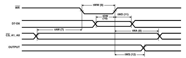
FIGURE 26. MODE 0 (BASIC OUTPUT)
