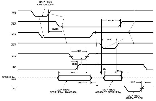
NOTE: Any sequence where  $\overline{\text{WR}}$  occurs before  $\overline{\text{ACK}}$  and  $\overline{\text{STB}}$  occurs before RD is permissible. (INTR = IBF • MASK •  $\overline{\text{STB}}$  •  $\overline{\text{RD}}$  +  $\overline{\text{OBF}}$  • MASK •  $\overline{\text{ACK}}$  •  $\overline{\text{WR}}$ )
