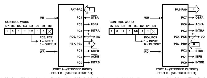
Combinations of Mode 1: Port A and Port B can be individually defined as input or output in Mode 1 to support a wide variety of strobed I/O applications.
