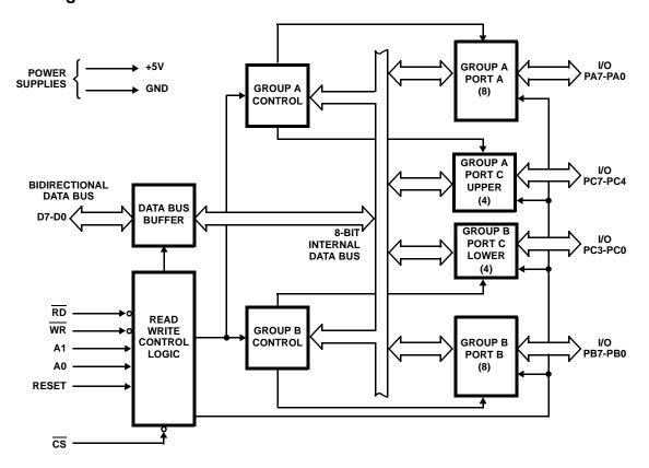
FIGURE 1. FUNCTIONAL DIAGRAM
