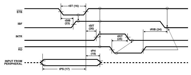
FIGURE 27. MODE 1 (STROBED INPUT)
