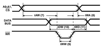
FIGURE 30. WRITE TIMING
