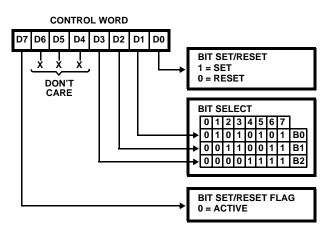
FIGURE 5. BIT SET/RESET FORMAT
