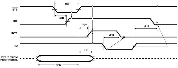
FIGURE 7. MODE 1 (STROBED INPUT)
