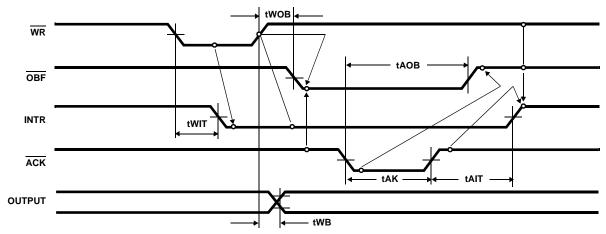
FIGURE 9. MODE 1 (STROBED OUTPUT)
