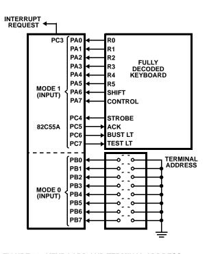
FIGURE 20. KEYBOARD AND TERMINAL ADDRESS INTERFACE
