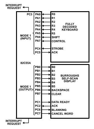
FIGURE 19. KEYBOARD AND DISPLAY INTERFACE
