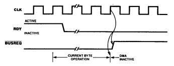
Figure 18. Bus Release When Not Ready (Burst Mode)
