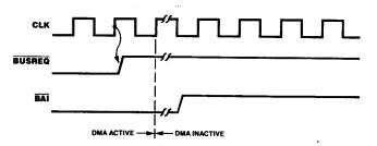
Figure 16. Bus Release (Byte-at-a-Time Mode)
