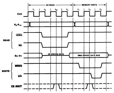
Figure 13. I/O-to-Memory Transfer
