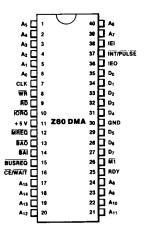
Figure 2a. 40-pin Dual-in-Line Package (DIP), Pin Assignments
