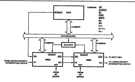
Figure 7. Multiple-DMA Interconnection to the Z80 CPU
