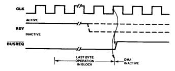
Figure 17. Bus Release at End of Block (Burst and Continuous Modes)
