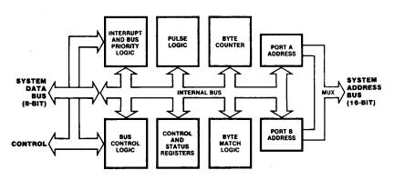
Figure 6. Block Diagram
