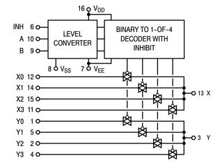
Figure 3. MC14052B Functional Diagram
