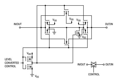
Figure 1. Switch Circuit Schematic
