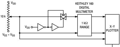
Figure 11. Channel Resistance (R<sub>ON</sub>) Test Circuit
