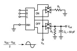
Figure 8. Channel Separation (Adjacent Channels Used For Setup)
