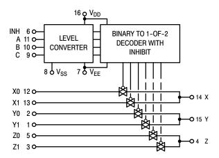
Figure 4. MC14053B Functional Diagram
