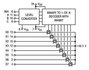
Figure 2. MC14051B Functional Diagram
