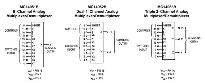
Note: Control Inputs referenced to  $V_{SS}$ , Analog Inputs and Outputs reference to  $V_{EE}$ .  $V_{EE}$  must be  $\leq V_{SS}$ .
