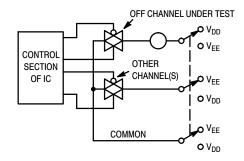
Figure 10. Off Channel Leakage
