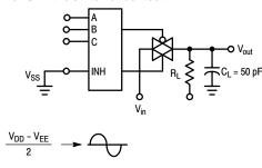
Figure 7. Bandwidth and Off-Channel Feedthrough Attenuation
