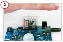
Stimulate the infrared sensor by moving your hand above the sensor.
