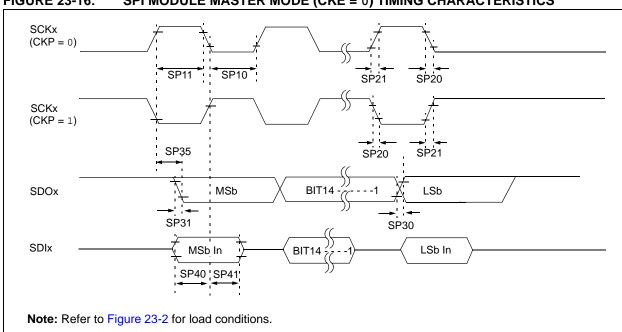
FIGURE 23-16: SPI MODULE MASTER MODE (CKE = 0) TIMING CHARACTERISTICS
