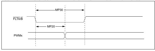
FIGURE 23-13: MOTOR CONTROL PWM MODULE TIMING CHARACTERISTICS
