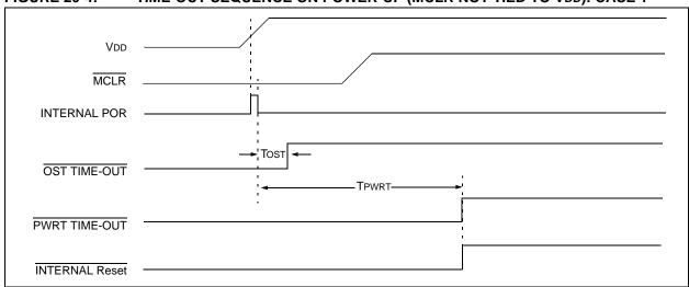
FIGURE 20-5: TIME-OUT SEQUENCE ON POWER-UP (MCLR NOT TIED TO VDD): CASE 2
