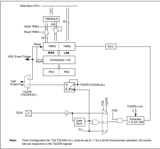
FIGURE 10-2: 16-BIT TIMER2 BLOCK DIAGRAM (TYPE B TIMER)
