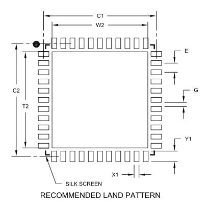
MILLIMETERS Units **Dimension Limits** MIN NOM MAX Contact Pitch 0.65 BSC Ε Optional Center Pad Width W2 6.80 Optional Center Pad Length T2 6.80 Contact Pad Spacing C1 8.00 Contact Pad Spacing C2 8.00 Contact Pad Width (X44) X1 0.35 Contact Pad Length (X44) <u>Y1</u> 0.80 Distance Between Pads G 0.25
