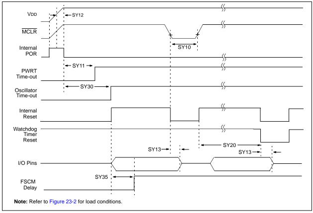
TABLE 23-20: RESET, WATCHDOG TIMER, OSCILLATOR START-UP TIMER, POWER-UP TIMER AND BROWN-OUT RESET TIMING REQUIREMENTS
