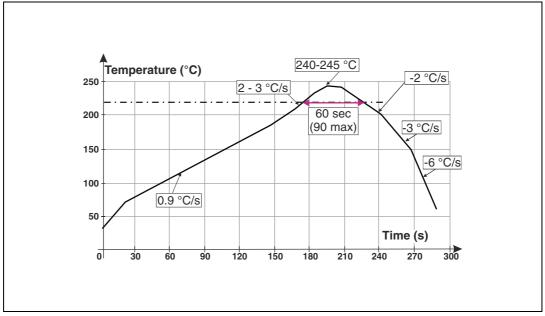
Figure 9. ST ECOPACK<sup>®</sup> recommended soldering reflow profile for PCB mounting
