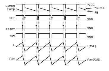
Fig.22 PWM switching timing chart
