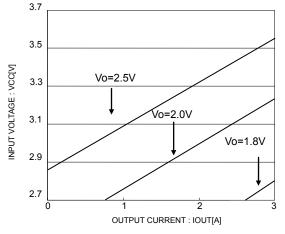
Fig.38 minimum input voltage in each output voltage
