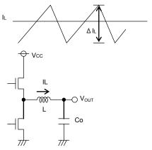
Fig.31 Output ripple current
