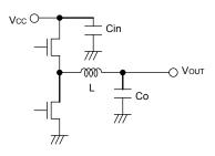
Fig.33 Input capacitor
