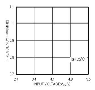
Fig.13 Power supply voltage-Operating frequency
