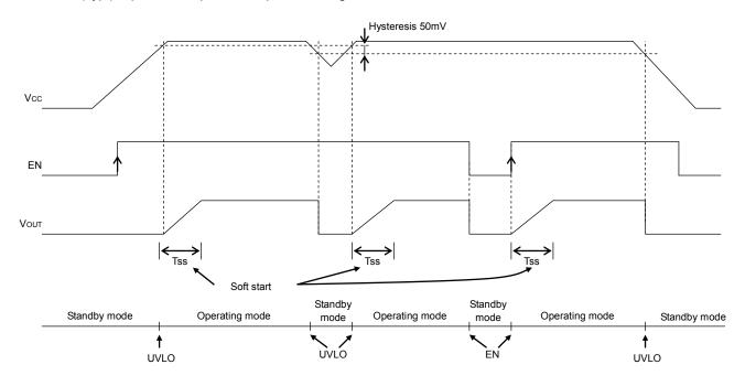
Fig.24 Soft start, Shutdown, UVLO timing chart
