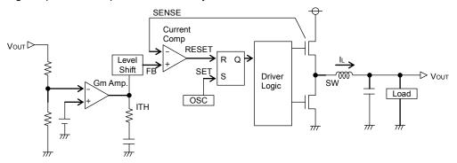
Fig.21 Diagram of current mode PWM control
