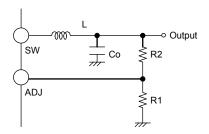
Fig.37 Determination of output voltage
