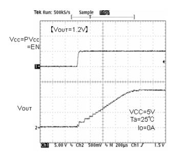
Fig.14 Soft start waveform
