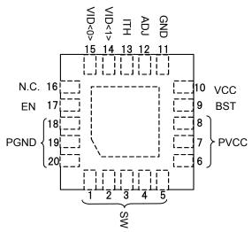
Fig.2 Pin configuration
