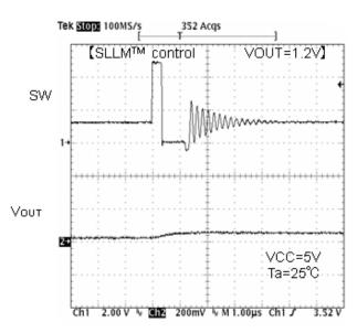
Fig.15 SW waveform Io=0mA
