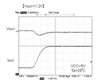
Fig. 17 Transient Response Io=1A→4A(20µs)
