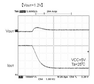
Fig.18 Transient Response Io=4A→1A(20µs)
