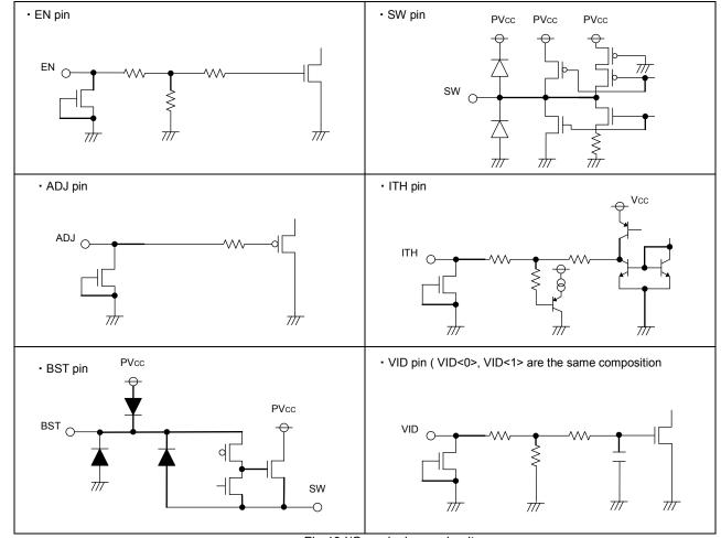
Fig.40 I/O equivalence circuit
