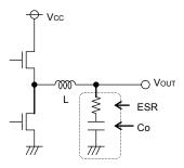
Fig.32 Output capacitor
