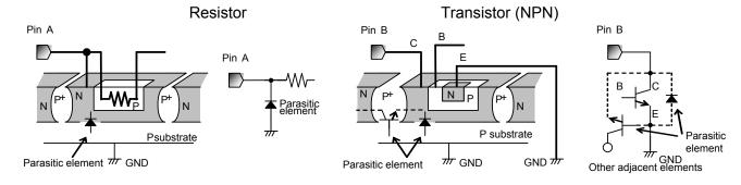
Fig.41 Simplified structure of monorisic IC
