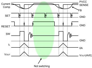
Fig.23 SLLM<sup>™</sup> switching timing chart
