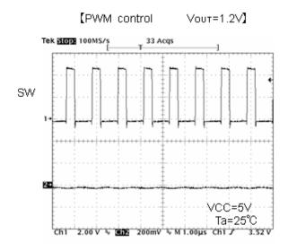
Fig.16 SW waveform Io=4A
