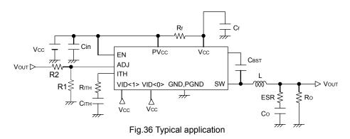
Stable feedback loop may be achieved by canceling the pole fp (Min.) produced by the output capacitor and the load resistance with CR zero correction by the error amplifier.
