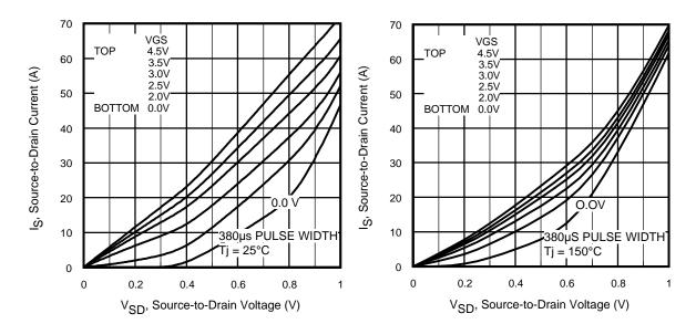
Fig 7. Typical Reverse Output Characteristics
