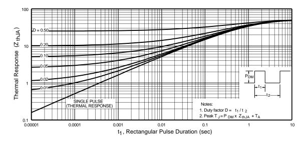
Figure 9. Maximum Effective Transient Thermal Impedance, Junction-to-Ambient
