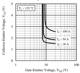
Figure 10. Collector-Emitter Voltage vs. Gate-Emitter Voltage
