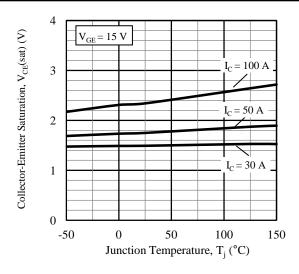
Figure 8. Saturation Voltage vs. Junction Temperature
