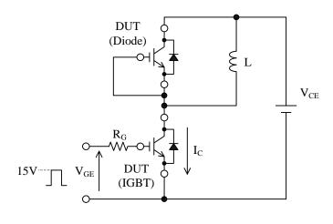
Test conditions  $V_{CE} = 300 \text{ V}$   $I_C = 50 \text{ A}$   $V_{GE} = 15 \text{ V}$   $R_G = 39 \Omega$   $L = 100 \ \mu\text{H}$
