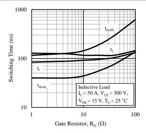
Figure 13. Switching Time vs. Gate Resistor
