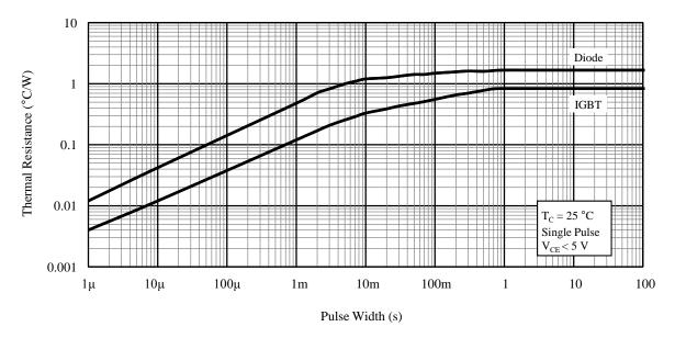
Figure 18. Transient Thermal Resistance
