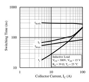
Figure 15. Switching Time vs. Collector Current
