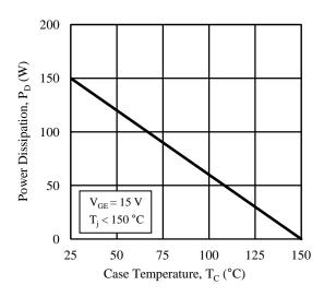
Figure 3. Power Dissipation vs. Case Temperature
