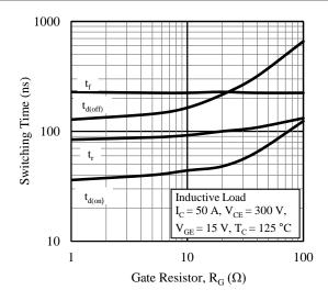
Figure 14. Switching Time vs. Gate Resistor
