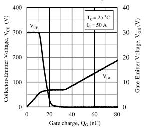
Figure 12. Gate Charge Characteristics
