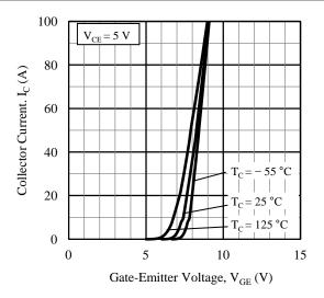
Figure 7. Transfer Characteristics
