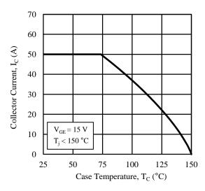
Figure 4. Collector Current vs. Case Temperature
