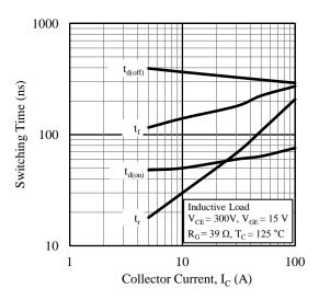
Figure 16. Switching Time vs. Collector Current
