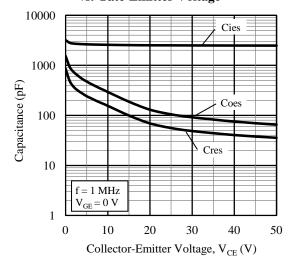
Figure 11. Capacitance Characteristics
