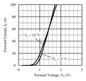
Figure 17. Diode Forward Characteristics
