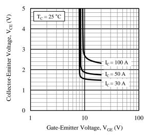
Figure 9. Collector-Emitter Voltage vs. Gate-Emitter Voltage
