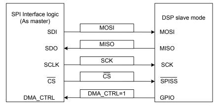
Figure-13 Master Mode (PIN\_DIR\_SEL=0)
