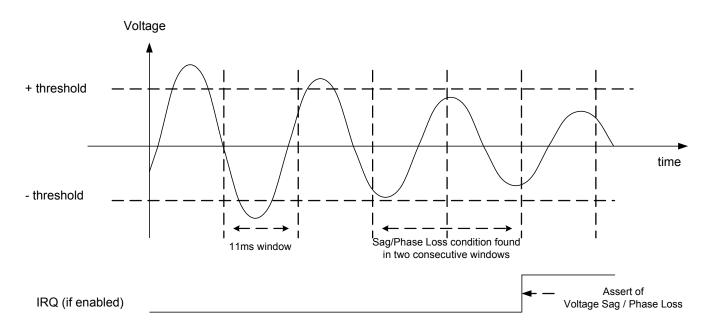
Figure-28 Voltage Sag and Phase Loss Timing Diagram
