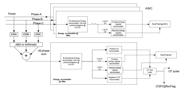
Figure-3 Energy Register Operation Diagram
