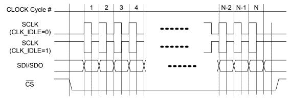
Figure-17 Clock Mode2 (CLK\_DRV=1, CLK\_IDLE=0) and Mode3 (CLK\_DRV=1, CLK\_IDLE=1)
