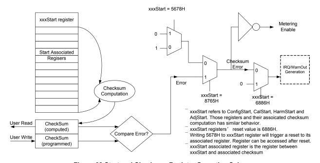
Figure-22 Start and Checksum Register Operation Scheme
