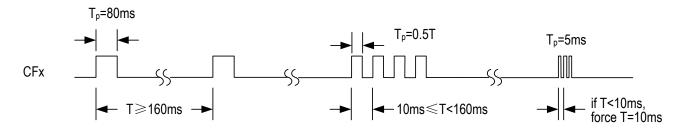
Figure-4 CFx Pulse Output Regulation
