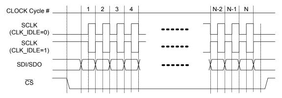
Figure-16 Clock Mode0 (CLK\_DRV=0, CLK\_IDLE=0) and Mode1 (CLK\_DRV=0, CLK\_IDLE=1)
