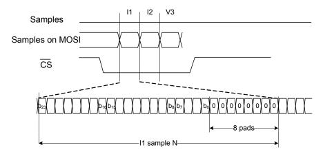
Figure-19 Sample Bit Sequence Example
