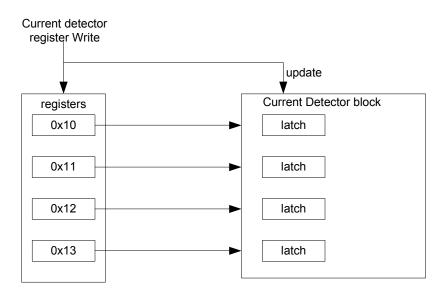
Figure-21 Current Detection Register Latching Scheme
