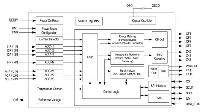
Figure-1 M90E36A Block Diagram
