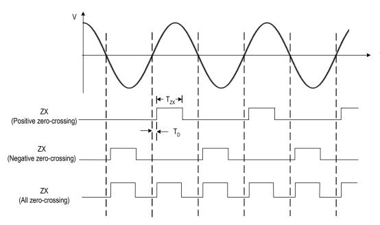
Figure-27 Zero-Crossing Timing Diagram (per phase)
