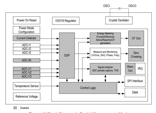
Figure-10 Block Diagram in Partial Measurement Mode
