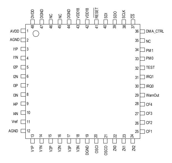
Figure-2 Pin Assignment (Top View)
