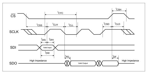
Figure-23 SPI Timing Diagram
