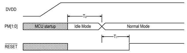
Figure-25 Power On Reset Timing (M90E36A and MCU are Powered on Simultaneously)
