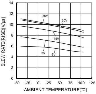
Figure 21. Slew Rate L-H - Ambient Temperature  $(RL=10k\Omega)$
