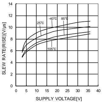
Figure 20. Slew Rate L-H - Supply Voltage  $(RL=10k\Omega)$
