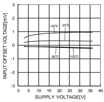
Figure 12. Input Offset Voltage - Supply voltage
