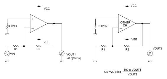
Figure 51. Test circuit 3 (Channel Separation)
