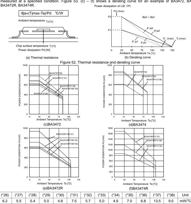
When using the unit above Ta=25°C, subtract the value above per degree°C.
