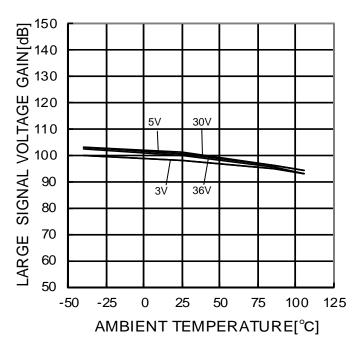
Figure 40. Large Signal Voltage Gain - Ambient Temperature
