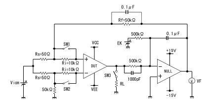
Figure 48. Test circuit 1 (one channel only)
