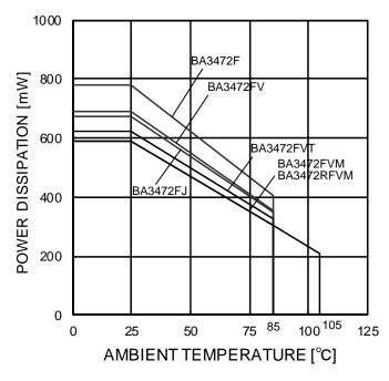
Figure 2. Derating Curve
