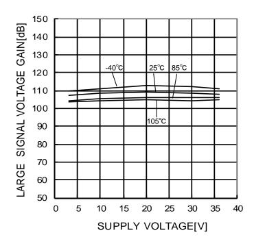
Figure 16. Large Signal Voltage Gain - Supply Voltage
