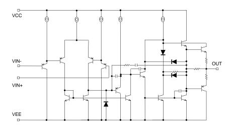
Figure 1. Simplified schematic (one channel only)
