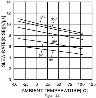
Figure 44. Slew Rate L-H - Ambient Temperature  $(RL=10k\Omega)$
