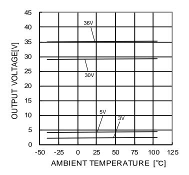
Figure 6. High level Output Voltage - Ambient Temperature (RL=10kΩ)
