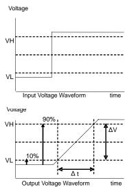
Figure 50. Slew rate input output wave
