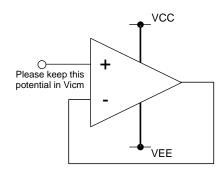
Figure 54. Unused circuit example
