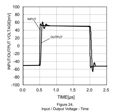
$RL=2k\Omega,\,CL=100pF,\,Ta=25^{\circ}C)$  (\*) The above data is measurement value of typical sample, it is not guaranteed.
