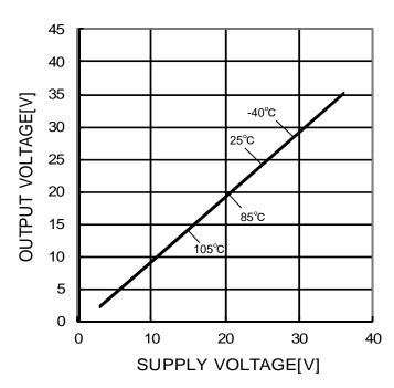
Figure 5. High level Output Voltage - Supply Voltage (RL=10kΩ)
