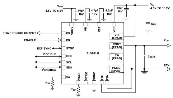
FIGURE 1. A COMPLETE DIGITAL SWITCH MODE POWER SUPPLY, ONLY BULK INPUT AND OUTPUT CAPACITORS ARE REQUIRED TO FINISH THE DESIGN
