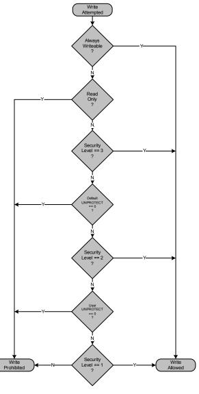
FIGURE 23. ALGORITHM USED TO DETERMINE WHEN A COMMAND IS WRITEABLE
