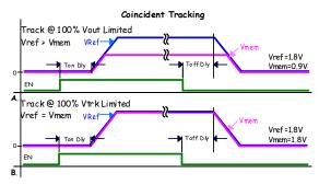
FIGURE 17. COINCIDENT TRACKING
