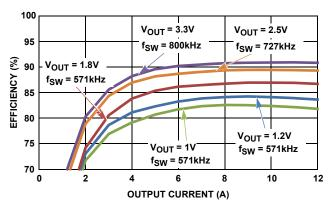
FIGURE 6. EFFICIENCY, VIN = 12V, FOR VARIOUS OUTPUT VOLTAGES
