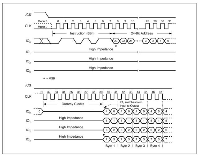
Figure 21. Fast Read Quad Output Instruction
