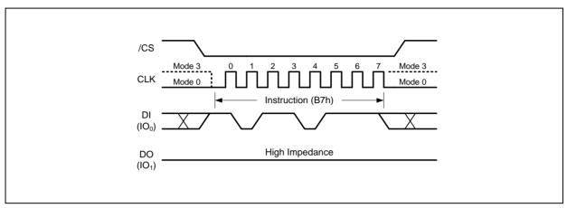
Figure 12. Enter 4-Byte Address Mode instruction
