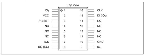
Figure 1b. W25M512JV Pin Assignments, 16-pin SOIC 300-mil (Package Code F)
