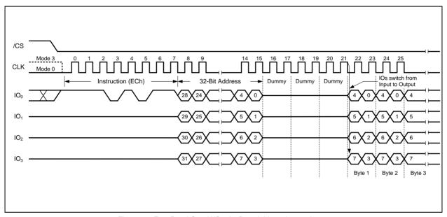
Figure 27. Fast Read Quad I/O w/ 4-Byte Address Instruction
