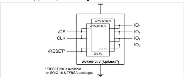
Figure 2a. W25M512JV Device Configuration
