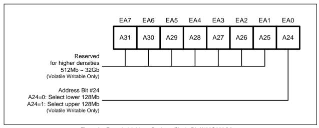
Figure 3e. Extended Address Register (Single Die W25Q256JV)
