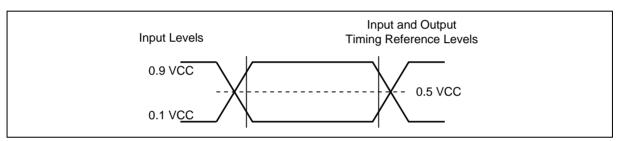
Figure 59. AC Measurement I/O Waveform
