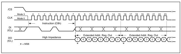
Figure 10. Read Extended Address Register Instruction
