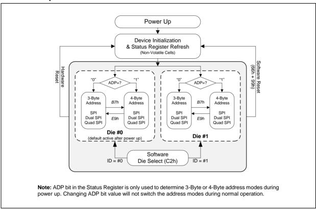
Figure 2c. W25M512JV Serial Flash Memory Operation Diagram
