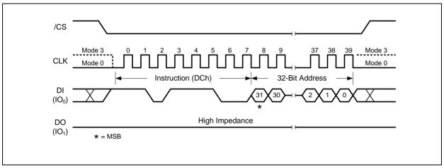
Figure 38. 64KB Block Erase with 4-Byte Address Instruction
