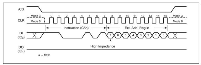
Figure 11. Write Extended Address Register Instruction
