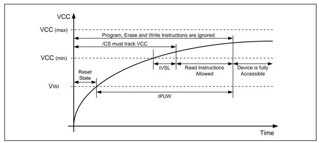
Figure 58a. Power-up Timing and Voltage Levels
