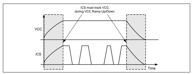
Figure 58b. Power-up, Power-Down Requirement
