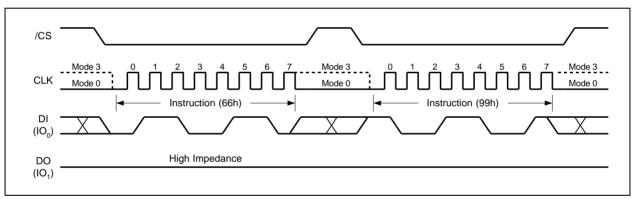
Figure 57. Enable Reset and Reset Instruction Sequence
