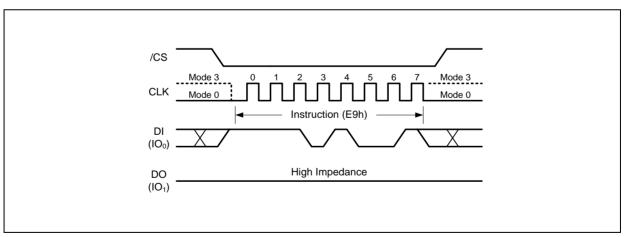
Figure 13. Exit 4-Byte Address Mode instruction
