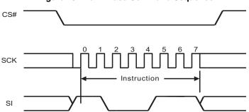
Figure 75. Bulk Erase Command Sequence
