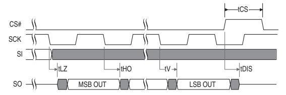
Figure 33. SPI SDR MIO Timing
