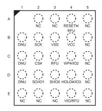
**Note:**Signal connections are in the same relative positions as FAC024 BGA, allowing a single PCB footprint to use either package.
