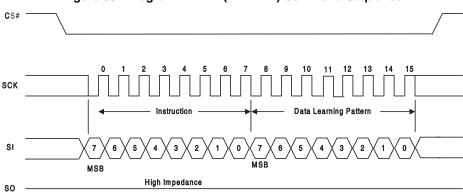
Figure 59. Program NVDLR (PNVDLR) Command Sequence
