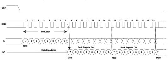
Figure 46. Read Bank Register (BRRD) Command
