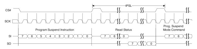
Figure 9.34 Program Suspend Command Sequence
