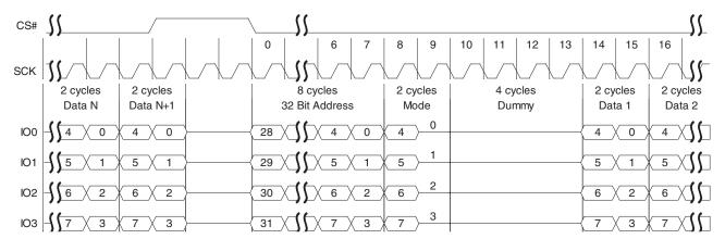
Figure 9.21 Continuous Quad I/O Read Command Sequence (4-byte Address), LC=00b
