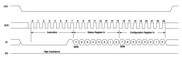
Figure 50. Write Registers (WRR) Command Sequence - 16 data bits
