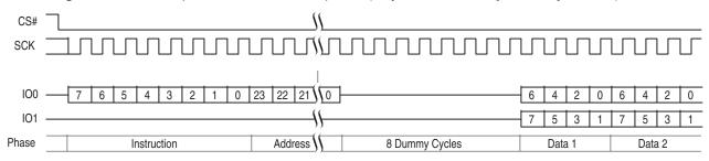
Figure 9.12 Dual Output Read Command Sequence (4-byte Address, 3Ch or 3Bh [ExtAdd=1, LC=10b])
