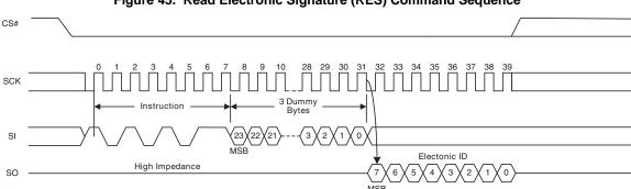
Figure 45. Read Electronic Signature (RES) Command Sequence
