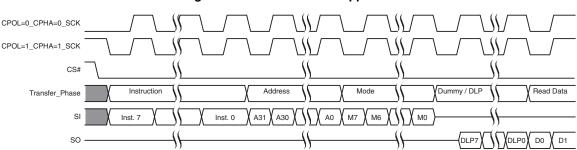
Figure 6. SPI DDR Modes Supported
