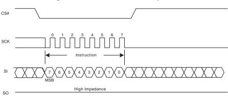
Figure 82. PPB Erase Command Sequence
