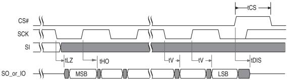
Figure 37. SPI DDR Data Valid Window
