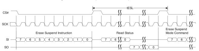
Figure 9.35 Erase Suspend Command Sequence
