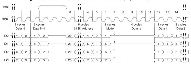
Figure 9.20 Quad I/O Read Command Sequence(4-byte Address, ECh or EBh [ExtAdd=1], LC=00b)
