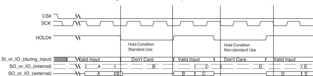
Figure 1. HOLD Mode Operation
