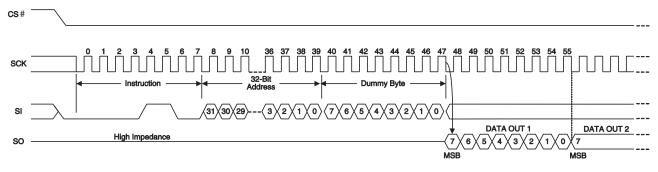
Figure 9.10 Fast Read Command Sequence (4-byte Address, 0Ch or 0B [ExtAdd=1], LC=11b)
