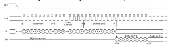
Figure 54. ECC Status Register Read Command Sequence
