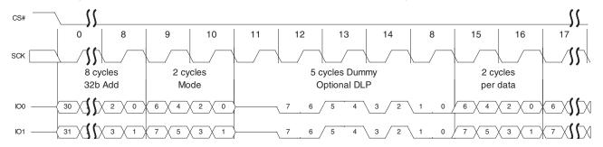
Figure 9.29 DDR Dual I/O Read (4-byte Address, BEh or BDh [ExtAdd=1], HPLC=00b)
