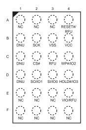
**Note:**1. Signal connections are in the same relative positions as FAB024 BGA, allowing a single PCB footprint to use either package.
