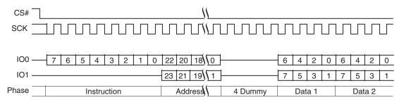
Figure 9.16 Dual I/O Read Command Sequence (4-byte Address, BBh [ExtAdd=1], HPLC=10b)
