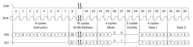
Figure 63. Continuous Dual I/O Read Command Sequence (4-byte Address, BCh or BBh [ExtAdd=1], EHPLC=10b)
