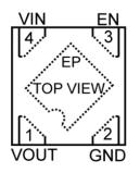
4-Pin 1mm × 1mm Thin DFN (MT)
