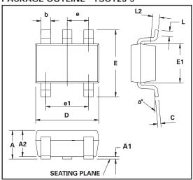
Controlling dimensions are in millimeters. Approximate conversions are given in inches
