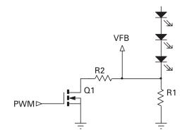
$$MOSFET 'off' \\ I_{LED(MIN)} = \frac{V_{FB}}{R_{LED}}$$
