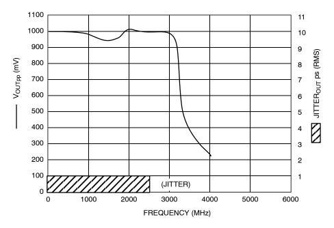
Figure 2. F<sub>max</sub>/Jitter
