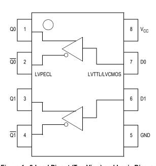
Figure 1. 8-Lead Pinout (Top View) and Logic Diagram
