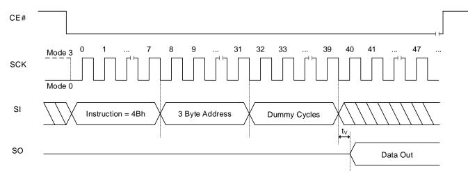
Note: Dummy cycles depends on Read Parameter setting. Detailed information in Table 6.11 Read Dummy Cycles.
