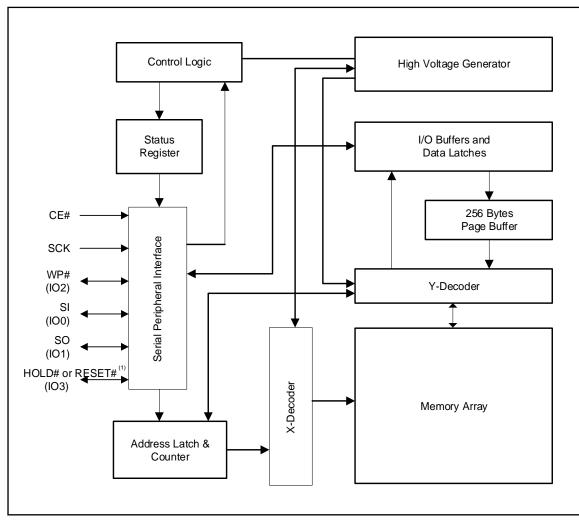
Note1: In case of 16-pin SOIC or 24-ball TFBFA, dedicated RESET# can be supported without sharing with HOLD# pin for the dedicated parts. See the Ordering Information for the dedicated RESET# option.
