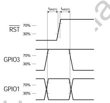
Figure 2. Reset Timing Parameters for Busmode Select Method 2 (GPIO3 = 1)
