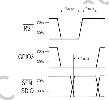
Figure 1. Reset Timing Parameters for Busmode Select Method 1 (GPIO3 = 0)
