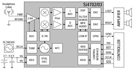
Figure 7. Si4702/03-D30 FM Receiver Block Diagram
