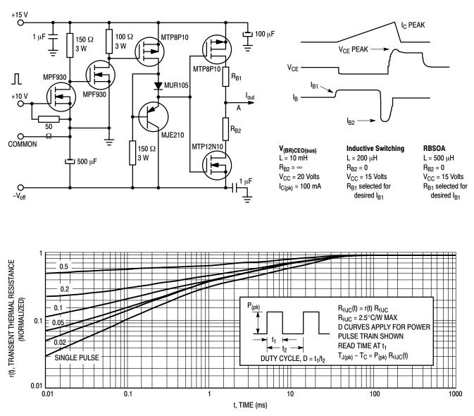
Figure 22. Typical Thermal Response ( $Z_{\theta JC}(t)$ ) for BUH50
