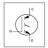
600 V  $I_{C(nom)} = 18A$   $V_{CE(on)} typ. = 1.65V @$   $I_{C(nom)} @ 25^{\circ}C$ Motor Control IGBT
