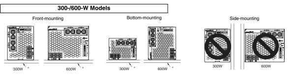
Note: 1. Improper mounting will interfere with heat dissipation and may occasionally result in deterioration or damage of internal parts. Use the standard mounting method only.
