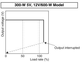
If an excessive current flows for 5 s or more, the output will be turned OFF and simultaneously the protection-ON alarm indicator will be lit. To reset the S8JX, turn OFF the power, leave the S8JX for at least three minutes, and then turn it ON again.
