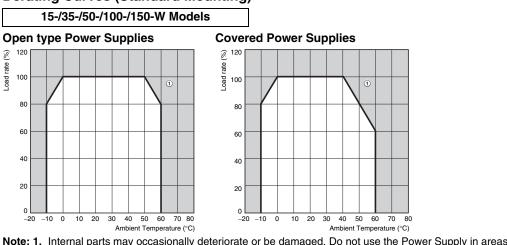
Note: 1. Internal parts may occasionally deteriorate or be damaged. Do not use the Power Supply in areas outside the derating curve (i.e., the area shown by shading ① in the above graph).
