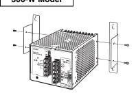
Note: To provide ventilation space, the body will shift forward by 21.6 mm from the mounting surface.
