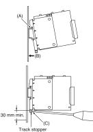
To dismount the Power Supply, pull down portion (C) with a flat-blade screwdriver and pull out the Power Supply.
