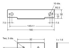
Note: Mounting Brackets are provided in a set, one for the right side and one for the left side.
