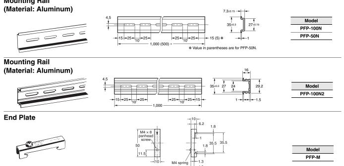
Note: 1. If there is a possibility that the Unit will be subject to vibration or shock, use a steel DIN Rail. Otherwise, metallic filings may result from aluminum abrasion.
