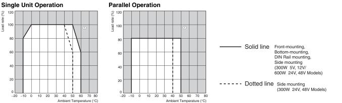
Note: 1. Internal parts may occasionally deteriorate or be damaged. Do not use the Power Supply in areas outside the derating curve (i.e., the area shown by shading (1) in the above graph). 2. If there is a derating problem, use forced air-cooling.
