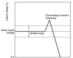
Note: Do not turn ON the power again until the cause of the overvoltage has been removed.
