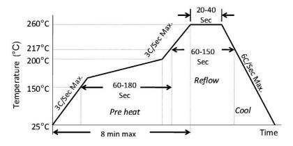
Figure 3. Solder Reflow Profile
