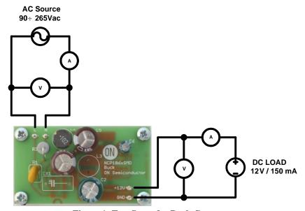
**Figure 1: Test Setup for Buck Convertor**
