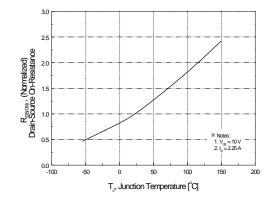
Figure 8. On-Resistance Variation vs Temperature
