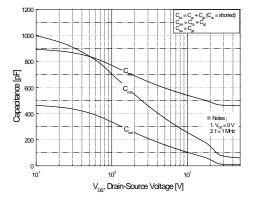
Figure 5. Capacitance Characteristics
