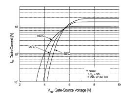
Figure 2. Transfer Characteristics
