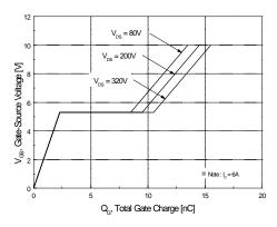
Figure 6. Gate Charge Characteristics
