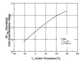
Figure 7. Breakdown Voltage Variation vs Temperature
