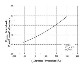
Figure 8. On-Resistance Variation vs. Temperature
