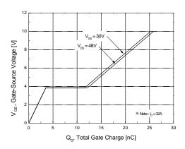
Figure 6. Gate Charge Characteristics
