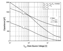
Figure 5. Capacitance Characteristics
