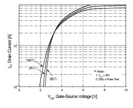
Figure 2. Transfer Characteristics
